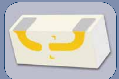
More conventional Al 2 O 3 Photo Diode Submount with side metallization. Thick film gold for wire bonding and palladium silver for soldering.
