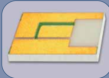
BeO Submount with plated copper and solder dams to prevent gold tin spreading. PCTF metallization exhibits consistent adhesion, whereas solder dams control die positioning.
